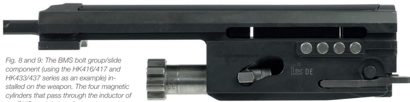
Fig. 8 and 9: The BMS bolt group/slide component (using the HK416/417 and HK433/437 series as an example) installed on the weapon. The four magnetic cylinders that pass through the inductor of the BMS module installed on the receiver during each movement of the bolt group/slide are clearly visible.
