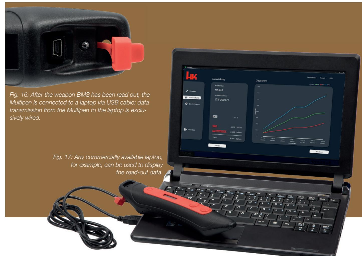
Fig. 16: After the weapon BMS has been read out, the Multipen is connected to a laptop via USB cable; data transmission from the Multipen to the laptop is exclusively wired.
