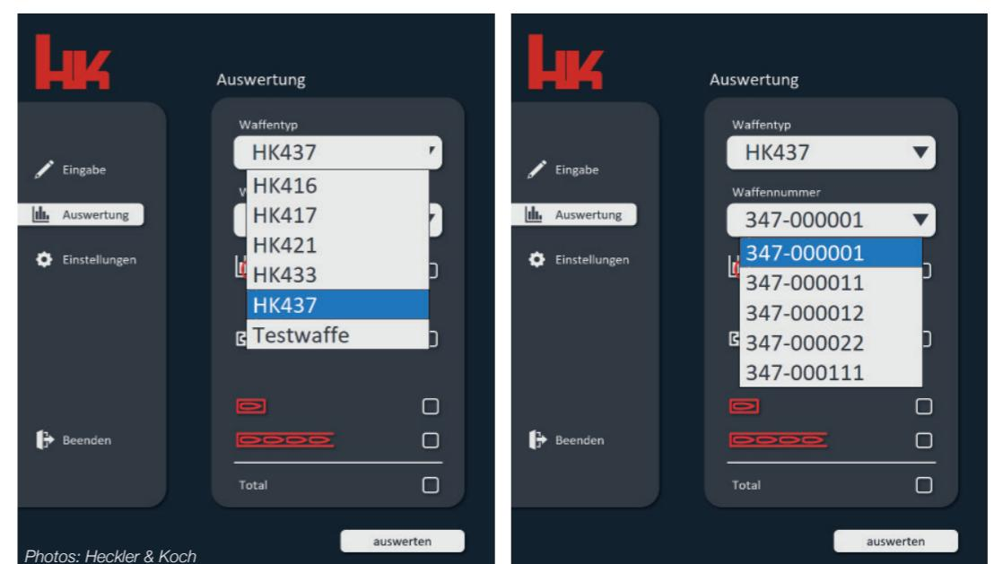
Fig. 18 and 19: Once the cable connection is established between the Multipen and laptop, the weapon model (left) and then its serial number (right) are selected from a drop-down menu in HK’s own display software. On the right, the boxes next to the pictograms can be clicked to display one, more than one or all three of the categories single fire, sustained fire and movements of the bolt group/slide with non-live rounds.
